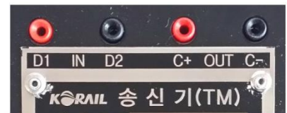
Front measurement terminal
